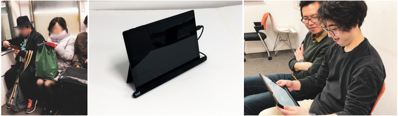
Figure 6: An application scenario for Private Reader (left). The current Private Reader prototype: a Surface Tablet with a Tobii 4C attached (mid) and a picture from the experimental setup (right).
