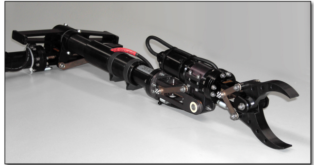
Fig. 2: The 123 dc-manipulator by sub-Atlantic which was used in our experimental setup.
