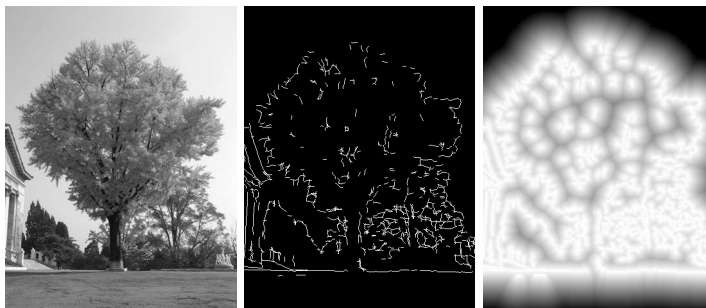
Fig. 5. Edge Image and Height Map. Left: original gray value image. Middle: binary edge image. Right: gray value height map. Note the gap in the top of the tree outline in the edge image. The height map compensates perfectly for this deficiency.
