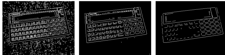
Fig. 3. Edge Images for Different Sets of Parameters. Left: \{d = 1, b = 1, \gamma = 2.0, \epsilon = 0.01, \lambda = 1.0\} . Middle: \{d = 1, b = 1, \gamma = 2.5, \epsilon = 0.01, \lambda = 1.0\} . Right: the same parameters as in fig. 2, i.e., \{d = 2, b = 2, \gamma = 3.0, \epsilon = 0.01, \lambda = 1.0\} .
