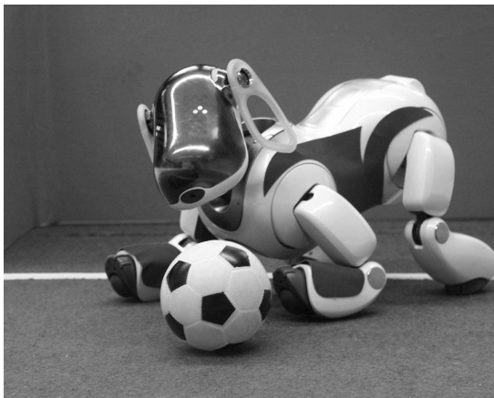
Fig. 1. Sony's ERS-7. This is the newest 20 degree-of-freedom, fully autonomous four-legged robot used in RoboCup robot soccer games.
