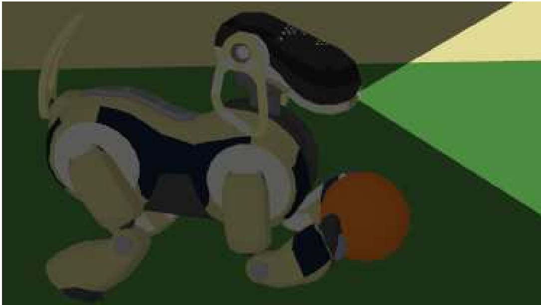
Figure 3.6: An Aibo which turns around a ball and cannot see it. To illustrate this the opening angle of the camera is lit.
