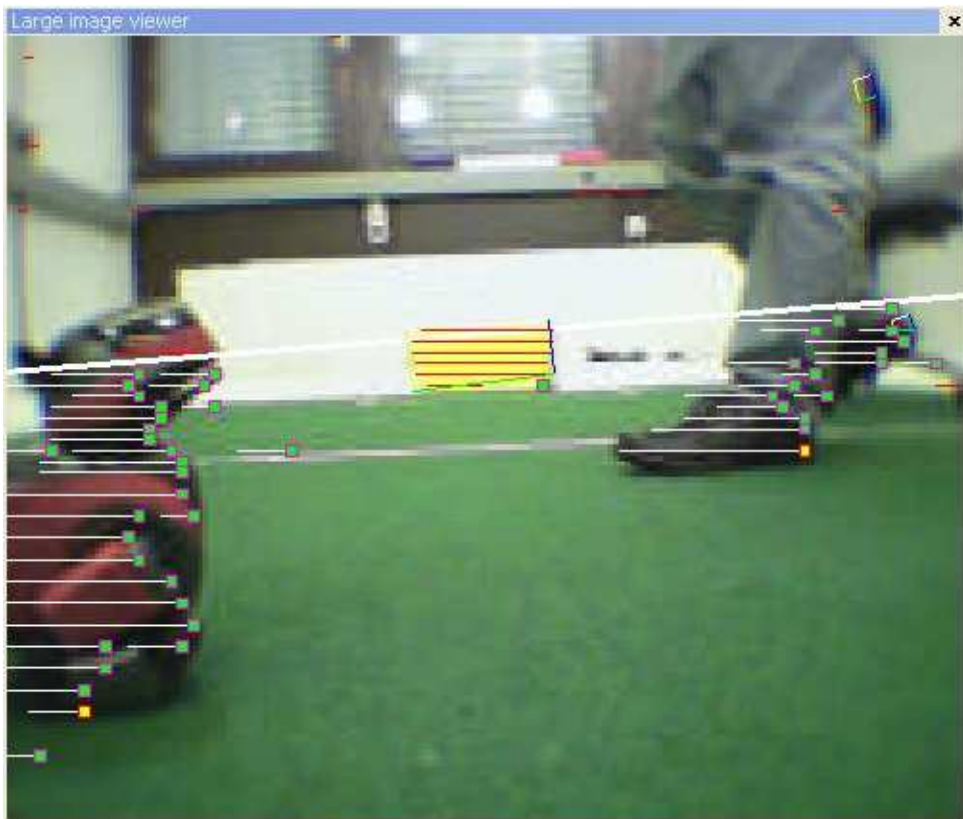
Figure 4.17: On the left a masked Sony Aibo ERS-210 is seen. The thick white line illustrates the horizon, whereas the thin white lines are the Line Pairs. A green point indicates the end of each Line Pair. A yellow point shows which point of the Line Pairs of a given cluster is taken as footpoint. Note that the two Line Pairs near the red Aibo (in its shadow and at the field line) do not belong to the cluster of the detected robot. However they are not recognized as own opponents due to their low validity.
