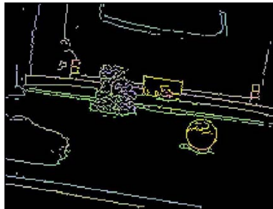
(d) filtered image with threshold hysteresis - Note, that the detected edge points hold some color information from the original image.
